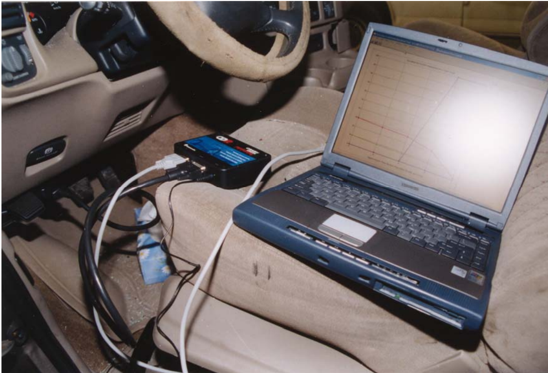
Photograph 3: A view of a Vetronix Crash Data Retrieval Tool and a notebook computer connected to the OBD link connector of a vehicle.
